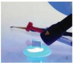
Fig. 1: Place Technovit fixing paste (page 15) on the bottom of the mounting mould. Fig. 2+3: Position specimen. Fig. 4: Cure fixing paste with the Technovit Blue LED. Embed specimen as usual.
