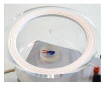
Draw vacuum in the Vacuum-Set, Technovit 2220 penetrates into any existing gaps
