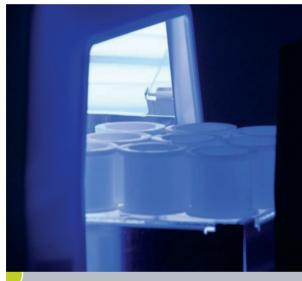
Homogenously illuminated specimen chamber with room for up to 9 specimens.
