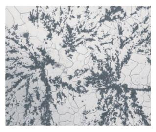
Original and impression of a mould. Ferritic grey cast iron with rosette-shaped arrangement of the graphite. Etched with 3% nitric acid.
